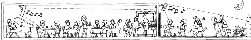
Figure 18. Piano Bar and Patio. LR4B used to project sound from main entertainment area. Weatherproof Musicasters used in outdoor patio system.
